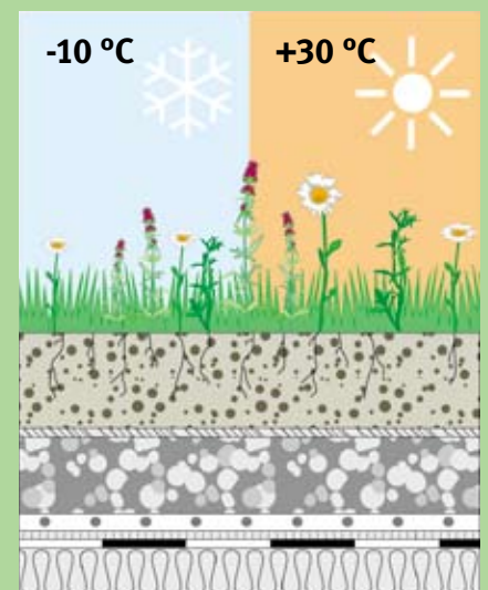
Thermal and mechanical protection of the waterproofing system
